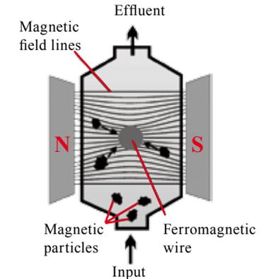
↑ Scheme of magnetic separation of small particles suspended in water flows
