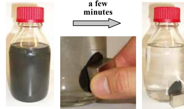
↑ Magnetic separation of magnetite nano-particles suspended as catalyst in water in the laboratory scale
