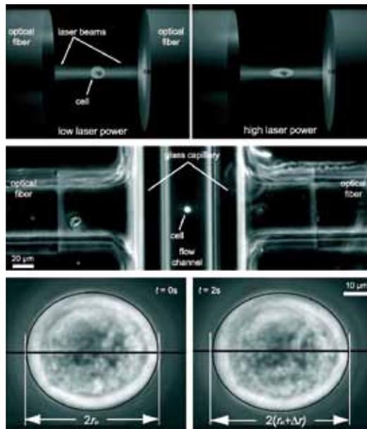
← The Optical Stretcher is a tool to probe viscoelastic properties of individual cells utilizing the pressure refracted light exerts on a surface. During a measurement cells are in suspension in a flow channel. Individual cells are trapped between two counter-propagating divergent laser beams emitted from opposing optical fibers. By increasing the laser power, the surface stress (due to the light pressure) increases and deforms the cell along the laser axis.
