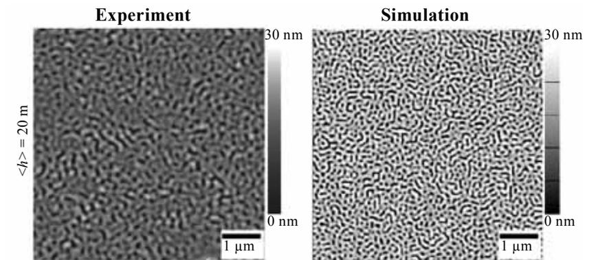
↑ Comparison of experiments (left) and computer simulations (right) on structure formation during vapor deposition of thin polycarbonate films on GaAs
