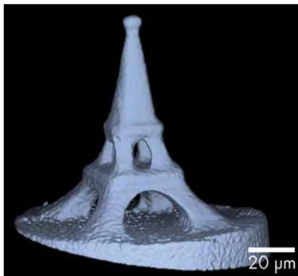
← Scanning transmission ion micro-tomogram of 3D architectural structure created by proton beam sculpting in PMMA
