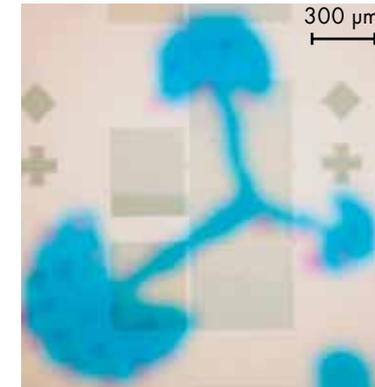
← Optical microscopic image of a fully transparent inverter circuit consisting of two MESFETs (background: laser-printed logo of BuildMoNa on an overhead transparency)
