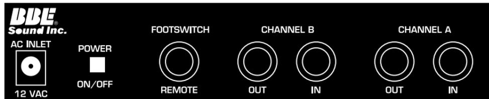
**6. A.C.INLET:** This jack is for connecting the 12 VAC power source.
