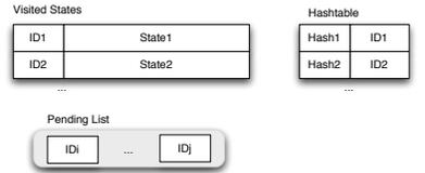
**Fig. 3.** Some Datastructures of the PROB Model Checker
